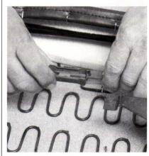
When you install the seat tracks, adjust the tracks by pushing both of them all the way back or forward. Tighten up the turnbuckle to a point where the seat-adjustment lever releases both seat tracks. Do not overtighten or the seat tracks will stay released.
