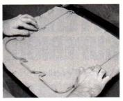
When your seats are stripped down, install new burlap material for "like-new" support. Do not forget to reinstall the wire structure shown here. Some folks leave it out, thinking it is unimportant. But this is what you're going to hog ring the new upholstery to.
