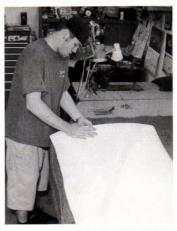
We see a lot of interiors with loose-fitting vinyl. There is a way around this. Mike Ambrose Custom Interiors in North Hills, California, lays down ½-inch layer of foam over the gauze material. This fattens up the seat, and makes it more comfortable to boot.
