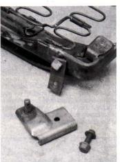
▲ In 1980, Ford did a recall addressing '68-'69 Mustang seatback failures. These failures were rooted in the inboard seatback pivot point. The fix is a bolt-on pivot assembly installed by drilling a hole and installing the new pivot, which is much stronger than original equipment.
