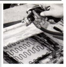
The '68-'69 seatback's foam arrangement differs from the '65-'67. This two-part foam block makes the seatback thicker. Don't be foolish and throw it away, thinking the aftermarket offers a reproduction. It doesn't. Use 3M Trim Adhesive to rejoin the two foam blocks.
