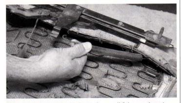
One of the most important seat tricks is protecting yourself. Before removing seat tracks, always carefully remove the helper spring, which will reduce the risk of injury from a runaway seat track.
