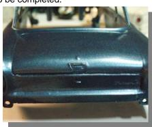
The next step in the conversion from a 61 to a 60 is removing the body mold trim and the Falcon emblem from the front fender. With that completed, we have to replace the lower trunk panel. The body is then sanded, painted and reassembled.
