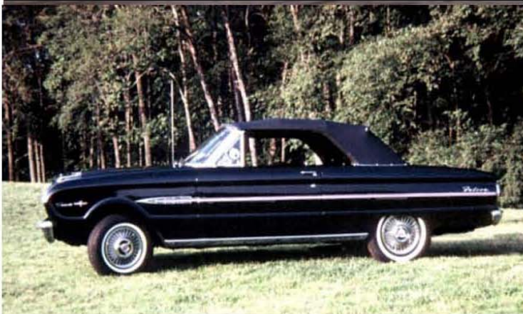
The Sprint in September of 1963, notice the larger 14" tires in the rear, while the front maintains the original 13"
