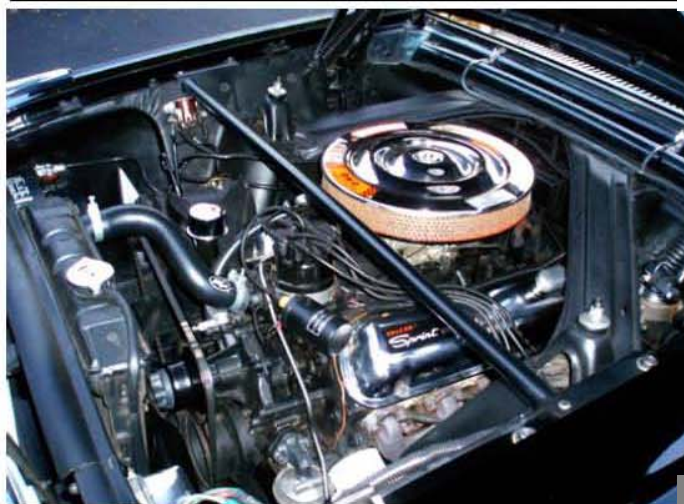
The engine is the original with a 289 Hi-Po 4 barrel and dual point distributor
