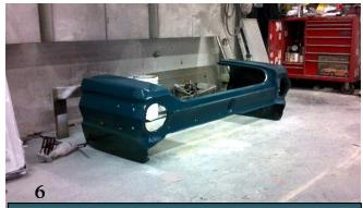
(6) I filled in the channel where the trunk weather-strip used to be. Then I painted it the same teal color as my Falcon.
