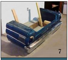
(7) The body was mounted on the frame and brackets made to hold the cushions.
