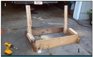
(1) I constructed a frame from 2×4s to hold the sheet metal.
