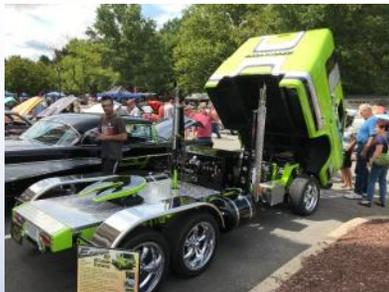
It began life as a '67 Econoline van. It was cut just behind the more forward of the two right side cargo doors. Then just the last few inches of the back of the truck were re-installed onto the body. My estimate is that approximately 3 to 4 feet of body were removed. The chassis is completely custom fabricated. The engine is a 351W. Power is driven through a T5 manual 5-speed transmission. The differential is from a Mustang. It has twin rear axles.
