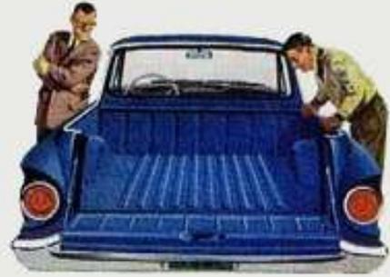
Low loading height. No strain here — level floor (no rear engine hump) measures just 25" to ground! Load capacity is 800 lbs., and Falcon's big 6-ft. box holds 8 ft. loads with tailgate flat. Use just one hand to open or close tailgate . . . it locks automatically!
