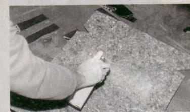
These sound-deadening pads not only keep out noise, they keep out heat and cold as well. Spray the trim adhesive, included in the kit, in liberal amounts on the back. Allow to tack off for five minutes. Then, lay it down.
