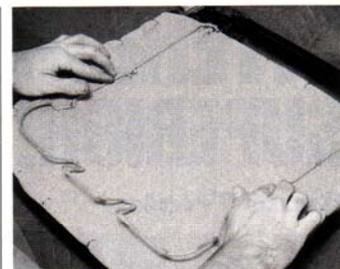
When your seats are stripped down, install new burlap material for "like-new" support. Do not forget to reinstall the wire structure shown here. Some folks leave it out, thinking it is unimportant. But this is what you're going to hog ring the new upholstery to.
