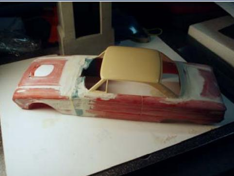
Step 4 - I started to fill the voids with modelers white putty.
