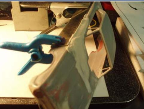
Step 7 - Now we apply putty to improve the contours. This time we used a straight edge to keep the lines more pronounced.
