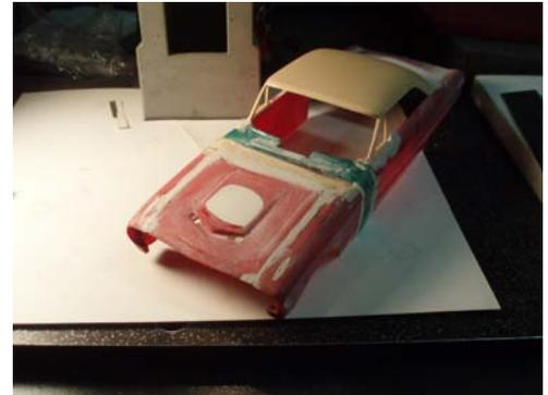
Step 3 - Now we cement the hood section to the car. I used Gorilla Super Glue for this.
