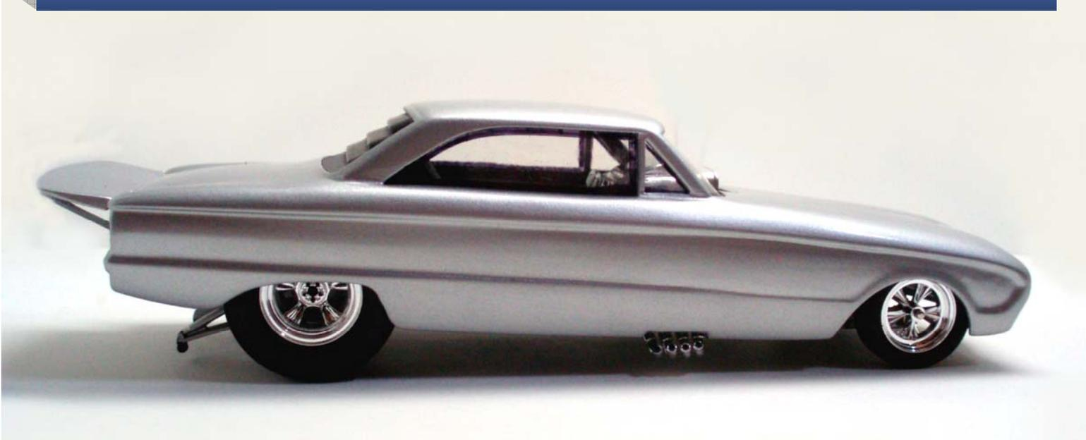
Step 12 - The car is now ready for the decals to be applied. It is washed in warm soapy water and rinsed with clean water and dried with a lint free towel. The decals are applied using Micro Set and Micro Sol setting solution for best adhesion and a painted on look.
