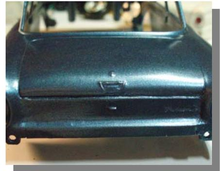
The next step in the conversion from a 61 to a 60 is removing the body mold trim and the Falcon emblem from the front fender. With that completed, we have to replace the lower trunk panel. The body is then sanded, painted and reassembled.
