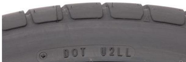
The use of a partial Tire Identification Number on the one sidewall (shown above) reduces the risk of injury to the mold technician that would have to install the weekly date code on the top sidewall portion of a hot tire mold.
